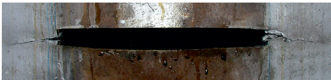
Fig. 15. TWC-controlled propagating shear evident in heavy-wall post-Millennial Grade 551 (X80) pipe
