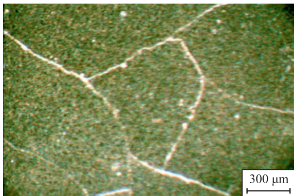
Fig. 1. Cracks on the surface of laser treatment zone (VK8 alloy) at energy density 2.0 J/mm 2 , treatment multiplicity 10
