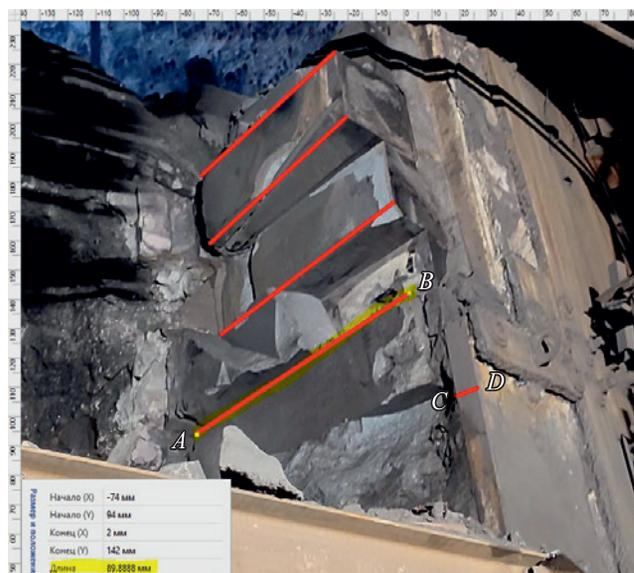
Fig. 6. Example of using the Visio tool to determine the residual linear size of a carbon refractory block (segment A – B) by scaling the known thickness of a cast iron stove (segment C – D)
