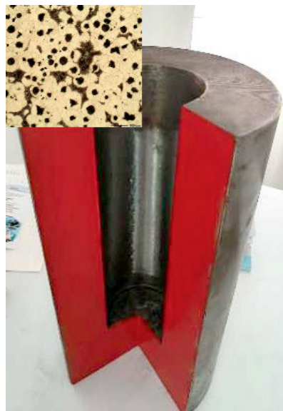
Fig. 2. Casting from high-strength ductile iron in the plant museum
