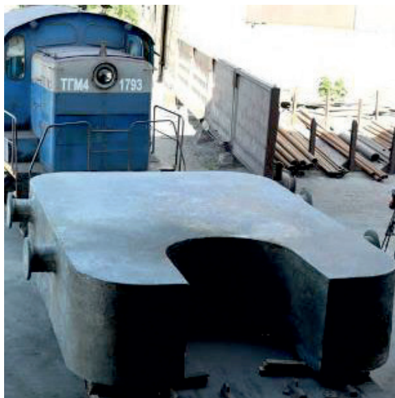
Fig. 3. Casting “anvil-block”, weight 87.5 tons
