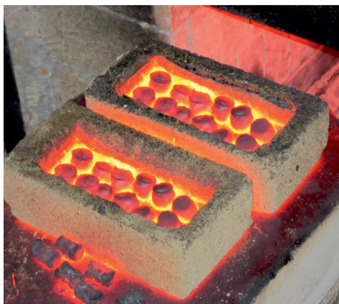
Fig. 5. Ore-coal briquettes during metallization in ceramic pallets
