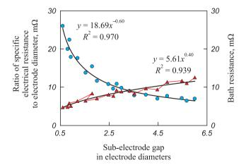
Changes in the bath active resistance and specific electrical resistance of the furnace melting zone depending on increase in sub-electrode gap when smelting 45 % ferrosilicon:
