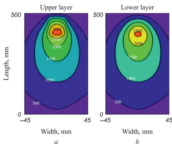
Fig. 3. Temperature distribution in the upper layer of a steel plate formed as a result of electric arc welding with (a) and without filler material (b)
