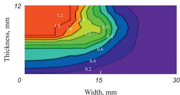
Fig. 7. Distribution of intensity of residual stresses located along the plate center thickness and formed as a result of automatic electric arc welding without filler material
