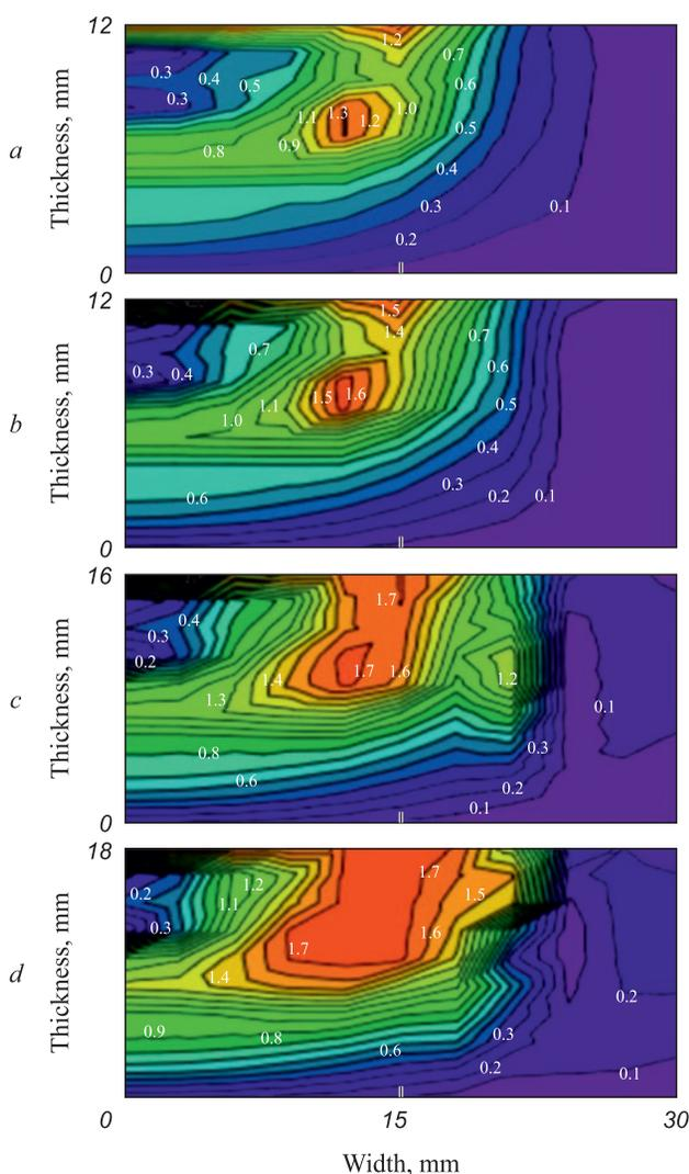
Fig. 6. Distribution of intensity of residual stresses located along the plate center thickness and formed as a result of automatic electric arc welding with aluminothermic backfill as filler material: 12 mm (*a*); 14 mm (*b*); 16 mm (*c*); 18 mm (*d*)
