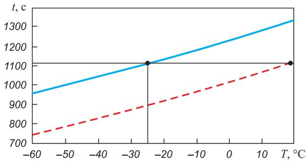
Fig. 4. Cooling time of a 12 mm thick plate
