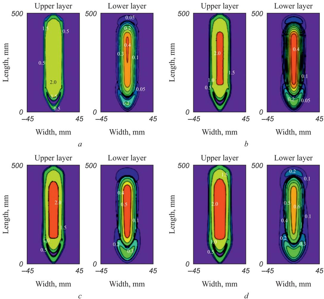
Fig. 5. Distribution of residual stresses intensity depending on plate thickness, formed as a result of automatic electric arc welding with filler material in the form of aluminothermic backfill: 12 mm (a); 14 mm (b); 16 mm (c); 18 mm (d)
