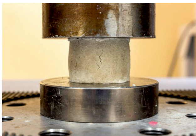
Fig. 3. Placing an experimental cylindrical sample in the testing machine during a compression test
