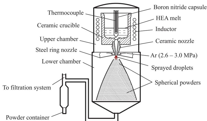
Fig. 3. Scheme of the unit for obtaining spherical powders by spraying the melt with inert gas
