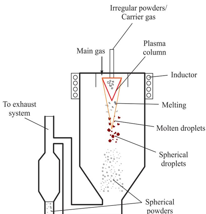
Fig. 2. Schematic diagram of plasma spheroidization system
