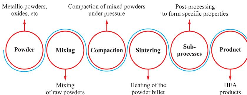
Fig. 1. Flow diagram of powder metallurgy
