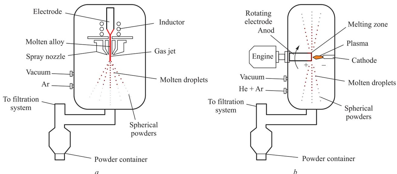
Fig. 4. Schematic diagrams of EIGA (a) and PREP (b) systems
