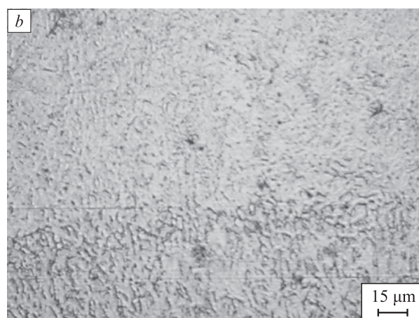
Fig. 5. Structure of sample 2 obtained by SLM: \times 200 (a); \times 500 (b)
