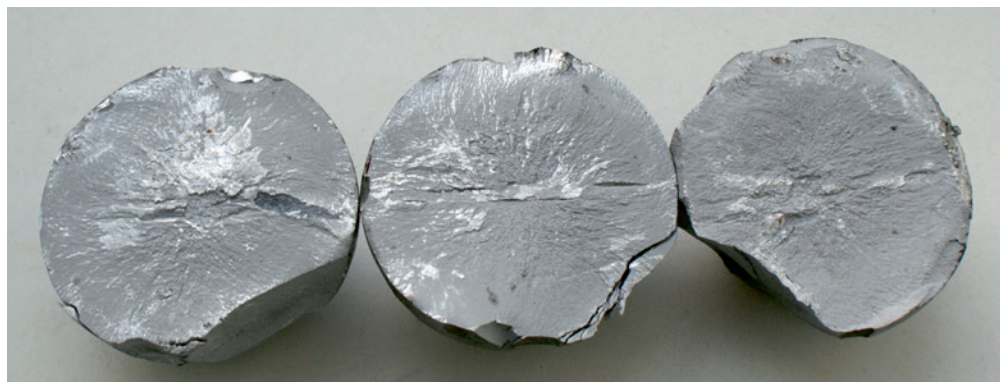
Fig. 3. Flakes in the balls fracture after impact resistance tests
